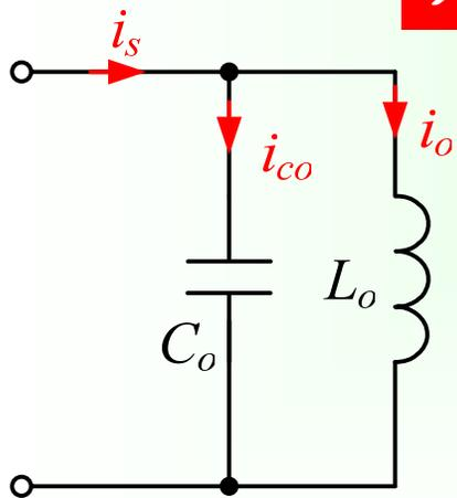
$$\zeta = \left| \frac{I_o(j\omega)}{I_s(j\omega)} \right| = \left| \frac{1}{1 - \omega^2 L_o C_o} \right|$$
