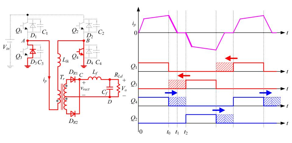
In order to ensure zero-current turn-off of the lagging switches, the turn-off time instant should be delayed to the time when  $i_p$  is reset or even to let the conducting time to be  $T_s/2$ .
