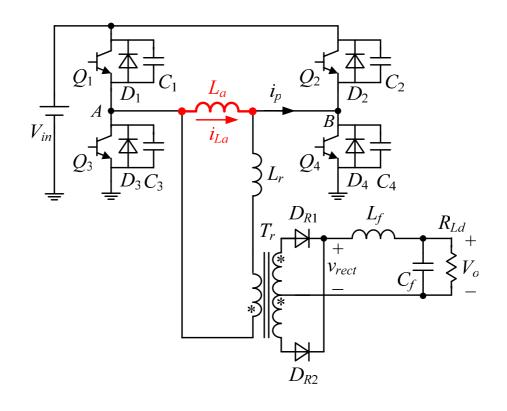
The auxiliary inductor current increases with the load current
