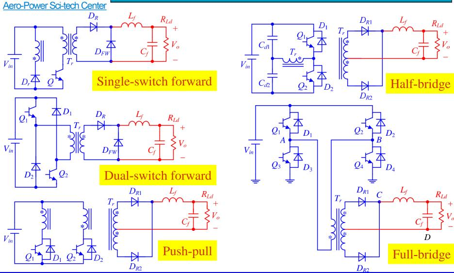
Among the buck-derived converters, the **full-bridge** converter can output **maximum power**, given that the power switches have the **same voltage and current ratings**.
