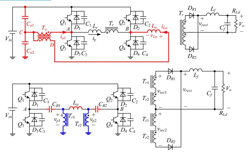
The auxiliary inductor current is adaptive with the load current, i.e., it is reduced as the load current increases.
