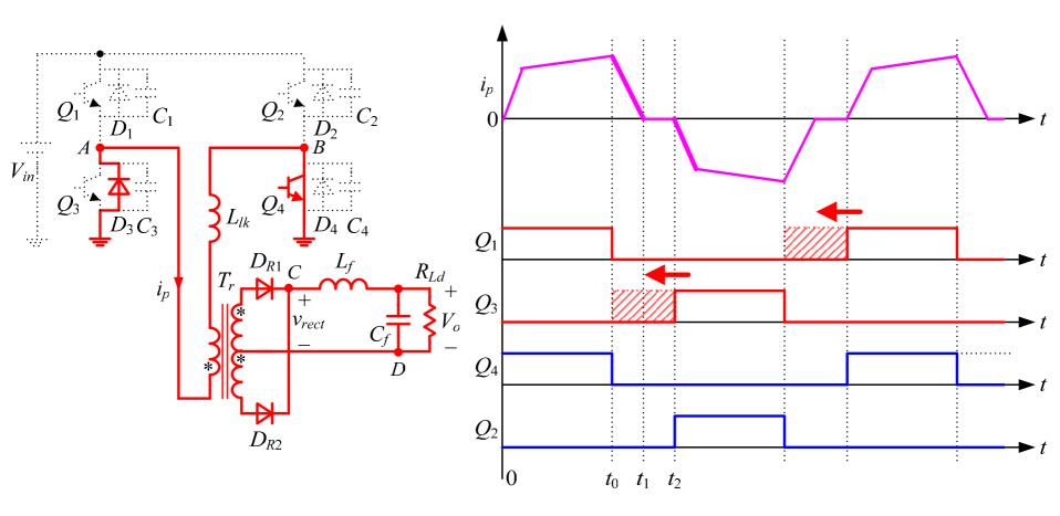
In order to ensure zero-voltage turn-on of the leading switches, the turn-on time instant should be moved forward and let the conducting time to be  $T_s/2$ .
