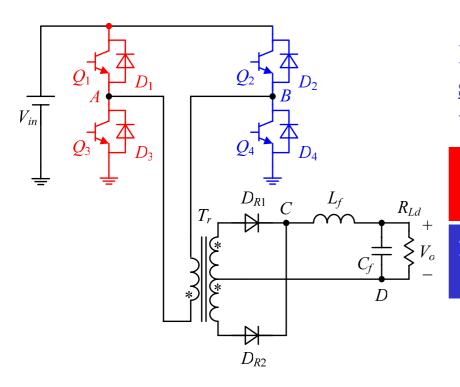
If the <u>turn-off instances</u> of the <u>diagonal</u> switches is staggered, the switching transition will be improved.
