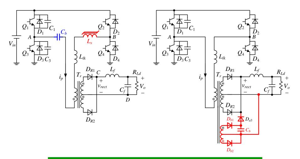
AB segment to block the reverse flowing path of  $i_p$
