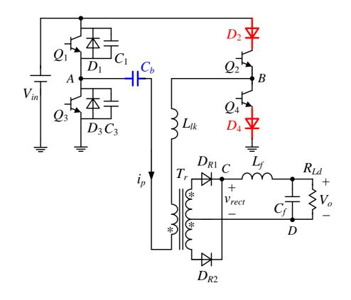
BC/BO segment to block the reverse flowing path of  $i_p$
