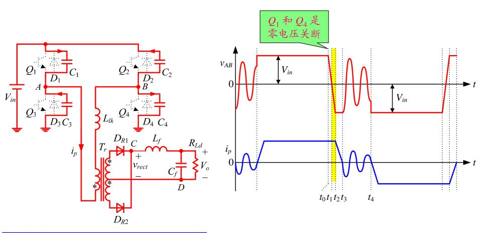
$v_A > v_B$  both the two rectifier diode conduct
