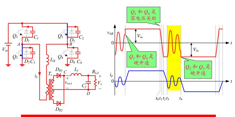
**Solution** If the diagonal switches turn off simultaneously, the power switches CAN NOT realize soft-switching.
