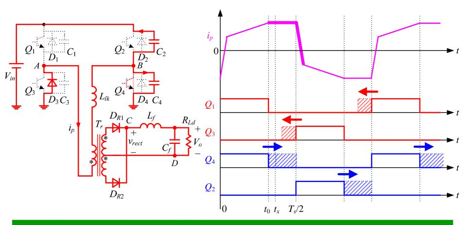
Since  $i_p$  flowing through the anti-paralleled diode of  $Q_3$  at zero state, the turn-on instant can be at any time, so the conduction time of the leading switches can be three kinds.
