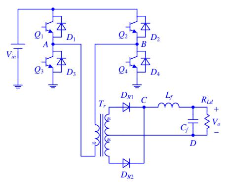
The full-bridge converter have widely used in medium-to-high power dc-dc conversions:
