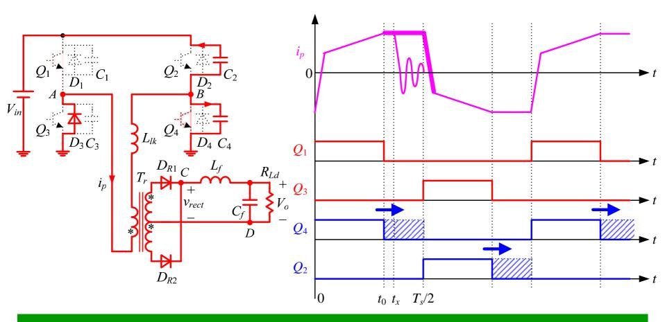
In order to ensure ZVS for the lagging switches, the turn-off time instant of the lagging switches should be delayed to  $T_s/2$ , i.e., the conducting time of the lagging switches should be  $T_s/2$ .
