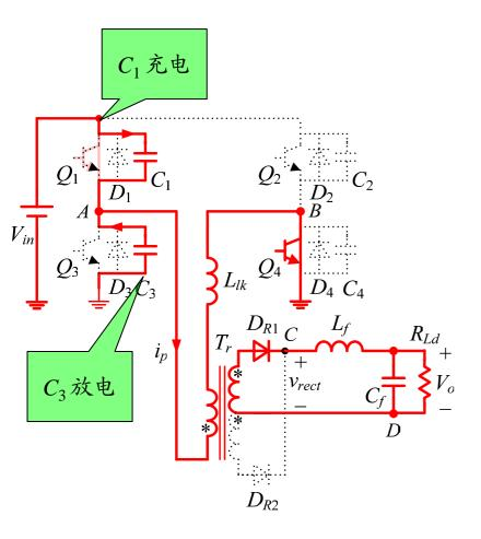
When the leading switch turns off, the current flowing out/into point A is the reflected output filter inductor current, a nearly constant current source.
